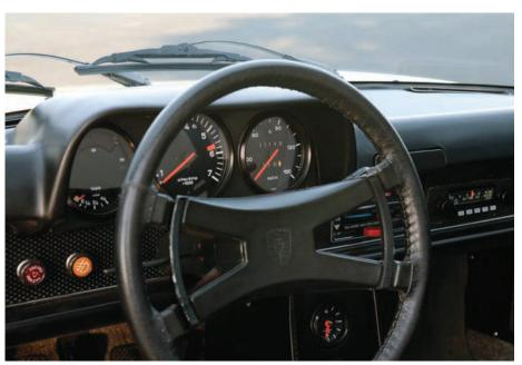
The 914 LE's gauges should look familiar to any Seventies Porsche aficionado, though the 914's speedometer only registers to 120 MPH instead of the 911's 150 MPH.
