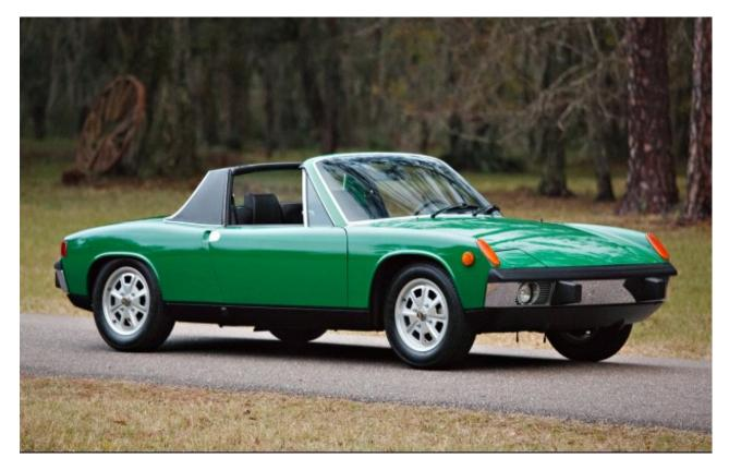
Jointly developed, manufactured, and marketed by Porsche and Volkswagen, the 914 was intended as the replacement for both the 912 and Karmann Ghia. Introduced in 1969, the well-balanced and surprisingly spacious Targa-topped roadster was equipped with an all-independent suspension, fuel injection, and five-speed gearbox as standard equipment. An enormous success, over 115,000 914 models were sold by the time production ceased in 1976.
