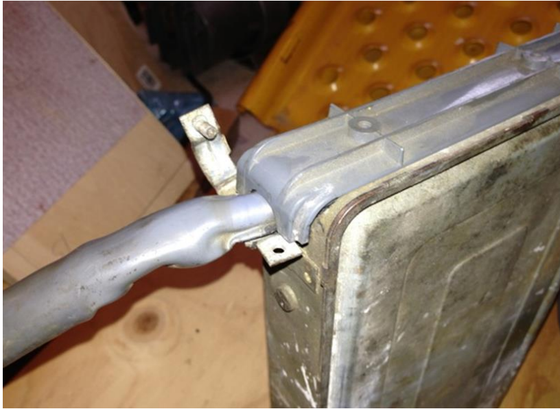
You will then be able to grab the plastic handle and unplug the harness from the ECU. Carefully pull it straight out
