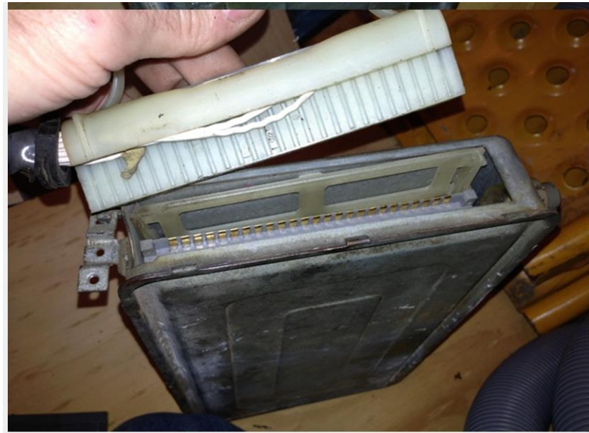
You will then be able to grab the plastic handle and unplug the harness from the ECU. Carefully pull it straight out
