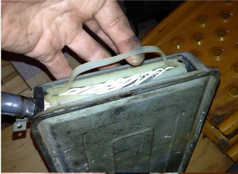
You will then be able to grab the plastic handle and unplug the harness from the ECU. Carefully pull it straight out
