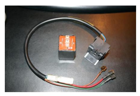
The wiper interval relay harness above (Fig. 2), includes a Relay-Socket with 5 female connectors, one in the center, 4 around. The 5 wires are color coded as follows: brown/black, blue/black, red, green/white, brown.
