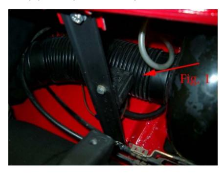
The relay socket mounts with one 6mm bolt/nut to the existing hole on the cowl brace (Fig 1)
