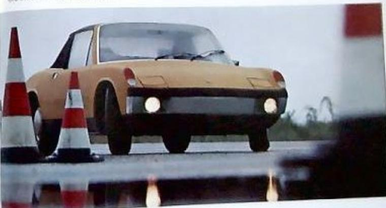
The 914/6 has a 2 litre, 110 HP six cylinder engine.
