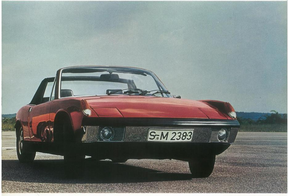
The rigid fiberglass roof of the Porsche (which incidentally saves you the money for a separate hardtop) can be removed in a few easy movements. In a matter of seconds the roof section can be stored in the rear luggage compartment. There it occupies only an inch or two of the usable luggage space.
