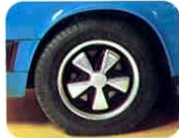
10. Forged Light Alloy Wheels. Lightweight 8-spoke wheels with Porsche Crest in relief. Open wheel design and weight reduction mean better
