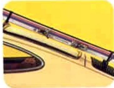
7. Ski Carrier. Made black, made of anodized aluminum. Holds two pairs of skis securely. Easily mounted and removed. When ordering, be sure to specify Porsche model.
