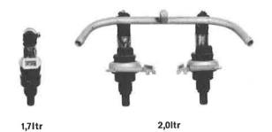
The injectors for the 2.0 liter engines have been given a larger opening gap. They are marked with a green plug socket. The injectors of the 1.7 liter engines are yellow.
