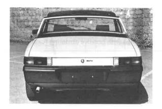
To increase ground clearance and assist the guide plates to dissipate excess heat under the vehicle, the rear apron has been shortened.
