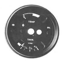
Basic equipment 2.0 liter vehicles are provided with a combined instrument containing an oil temperature gauge.
