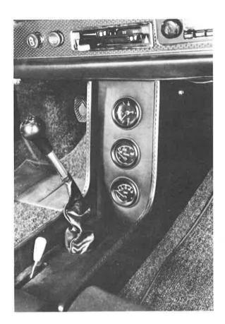
For the Porsche 914/2.0 liter a center console is offered. The console houses a clock, an oil temperature gauge and a voltmeter (battery). The gear shift lever is provided with a
