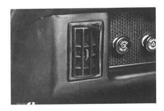
The lateral defroster nozzles are now equipped with a lever in place of the previously used knurl (for lateral adjustment) in order to simplify the operation.
