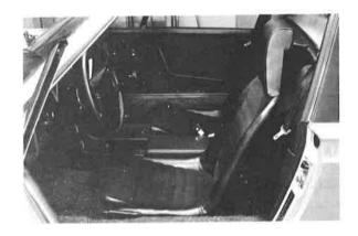
The longitudinal seat adjustment of the two seats in forward direction was reduced.
