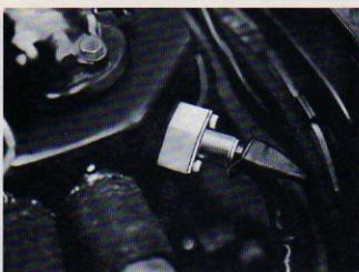
Start the engine and allow to idle. Loosen the lock nut at the pressure regulator and set the pressure to 2.0 + 0.05 kgf/cm2 (28.5 + 0.7 psi) by means of the hexagon head screw.
