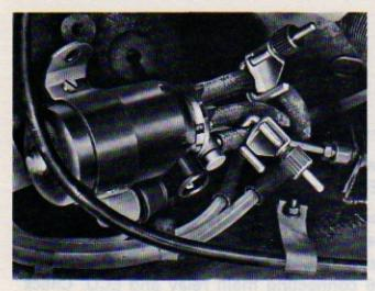
After the fuel pump has been installed, when connecting the fuel lines make sure that they are on no account interchanged!
