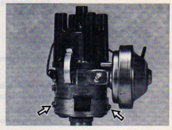
Before installing a new holder lubricate the sliding heels very lightly with Ft 1 v 4.
