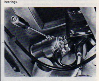
Open hose clamps of pressure, return and suction lines at fuel pump.
