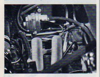
Temperature sensor II is located between the intake tubes.
