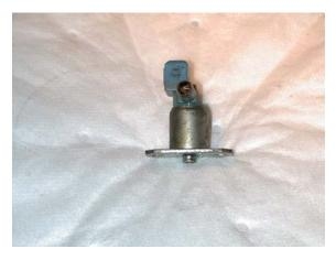
• Thermo-Time Switch – Located just below the cold start valve underneath the intake pipe on the passenger's side. It is distinguished by its long copper sensor.
