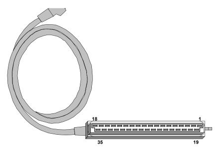
the top row of the plug has more pins and is longer than the bottom row. The following table may assist in using the Electronic Control Unit connector plug for measurement purposes.
