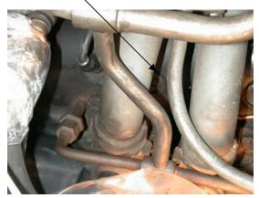
• Throttle Valve Switch – Located on the flywheel side of the throttle valve. The cover is removed in this photograph to illustrate the simple contact switch which senses the wide open throttle (WOT) condition only.
