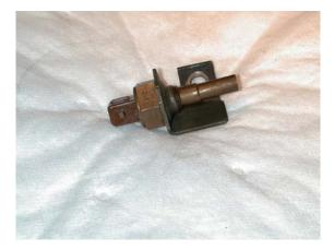
• Pressure regulator – This component is located below the air filter box along the back of the engine tin. Two fuel lines and the vacuum hose attachment allow easy recognition of this component.
