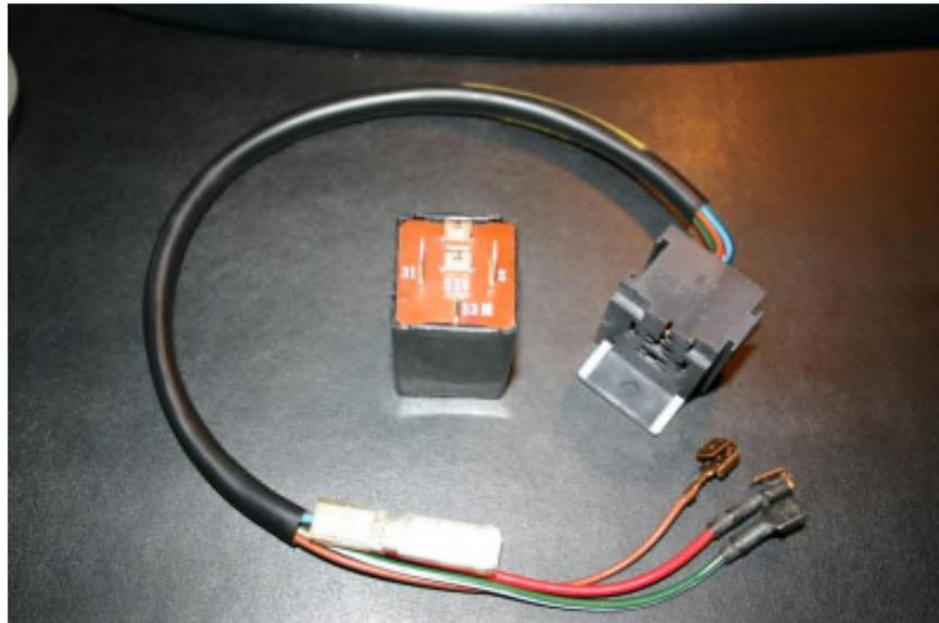
The wiper interval relay harness above (Fig. 2), includes a Relay-Socket with 5 female connectors, one in the center, 4 around. The 5 wires are color coded as follows: brown/black, blue/black, red, green/white, brown.
