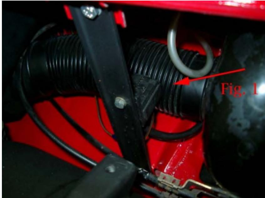
The relay socket mounts with one 6mm bolt/nut to the existing hole on the cowl brace (Fig 1)
